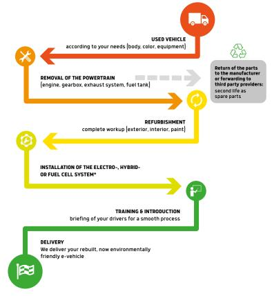
\*(depending on the type of drive, the corresponding components such as motor, batteries, power electronics, fuel cell, hydrogen tanks are installed)
