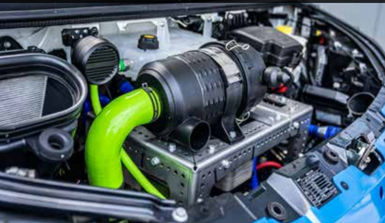
View of the engine compartment with fuel cell
