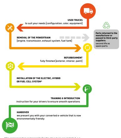
\*the corresponding components for the drive type are installed, e.g., e-motor, batteries, power electronics, fuel cell, hydrogen tank
