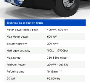
Concept Demo is 110kWh. 200 kWh solution available 2Q 2023
